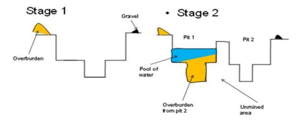
Figure 12: Drawings that illustrates how to perform the pitting method.
