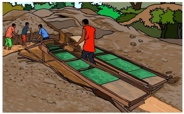
The concentrate on the mat is washed into a big tub, and the cycle is then usually repeated.
