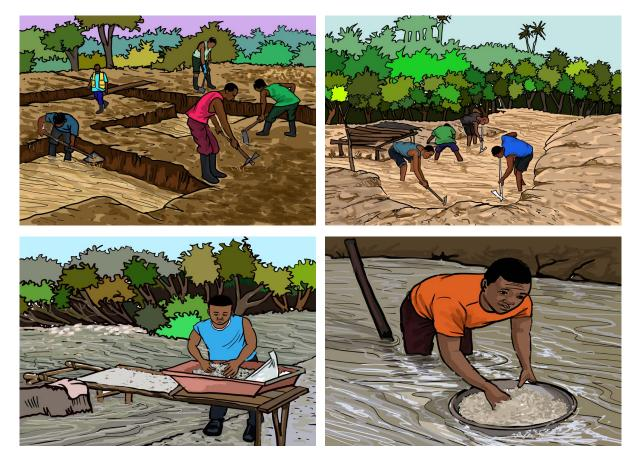
Figure 1: Picture showing so called "gold boys" (mine workers) digging pits, digging gravel, washing gravel, washing sluice box residue (clockwise from top left).
