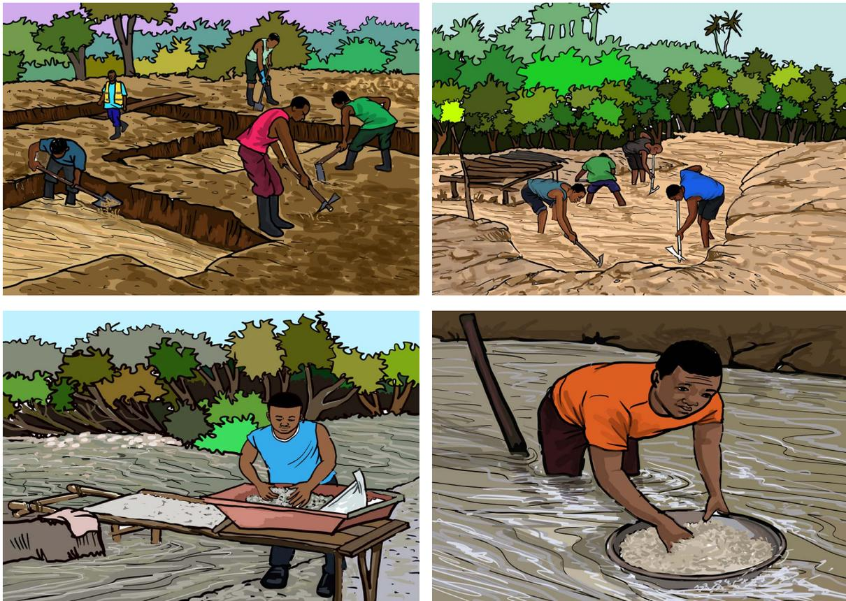
Figure 1: Picture showing so called “gold boys” (mine workers) digging pits, digging gravel, washing gravel, washing sluice box residue (clockwise from top left).
