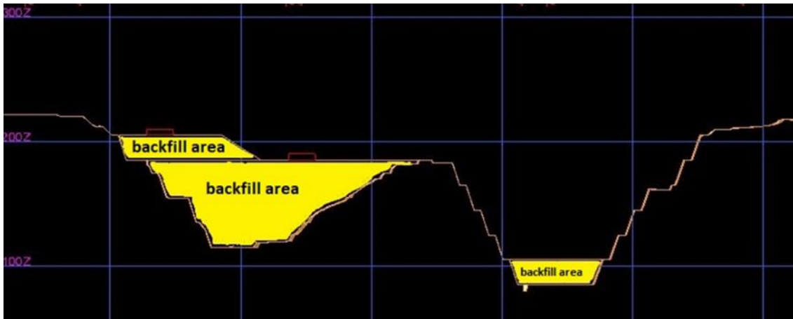
Figure 36 North-south cross-section of the open pit (at the End of Life of the mine, Arhavi Pit at the left will be backfilled almost completely. and Adana Pit at the right will be backfilled partly)
